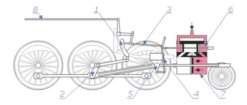
The main moving parts of a steam locomotive with Walschaerts valve gear: 1 - Link, 2 - Eccentric crank, 3 - Radius rod, 4 - Lap/lead lever, 5 - Crosshead, 6 - Valve, 7 - Cylinder, 8 - Reach rod
