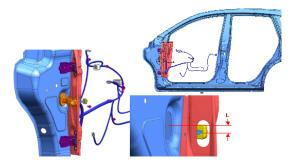
Fig. 2 Door structure and wiring harness(W/H) system
