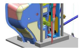
(a) 3D model simulation for slam tester
