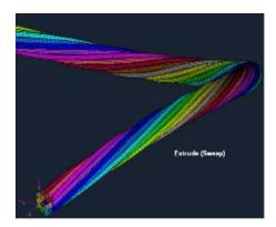
(a) Wire twist model with contact condition
