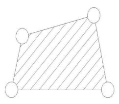
A mechanism is made of a number of resistant bodies out of which some may have motions relative to the others. A resistant body or a group of resistant bodies with rigid connections preventing their relative movement is known as a link.
