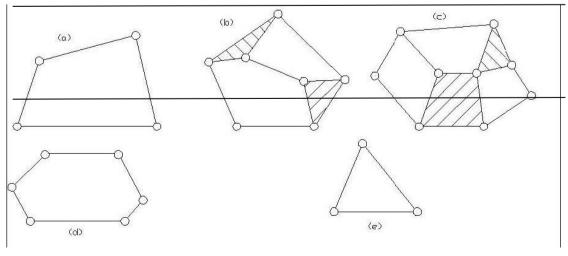
In case, the motion of a link results in indefinite motions of other links, it is a non-kinematic chain. However, some authors prefer to call all chains having relative motions of the links as kinematic chains.
