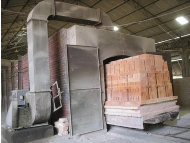
Fig - Tunnel Kiln Car loaded with Wares (Refractory Bricks) coming out of the Kiln after Firing.
