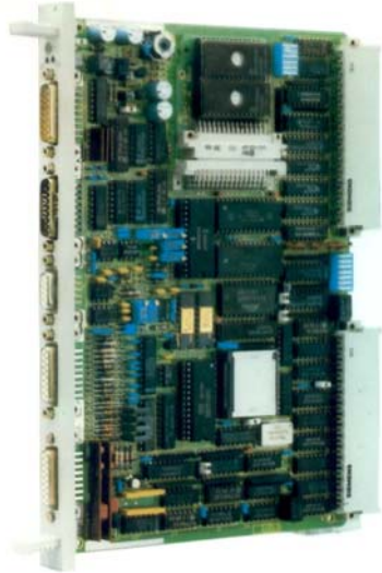
Fig. 36.1 Embedded Single Board Position Controller Module
