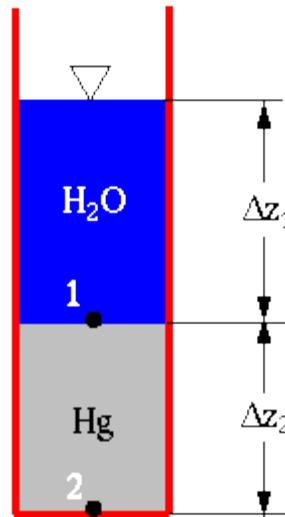
In this case, our hydrostatics equation must be used twice, once in each of the liquids.
