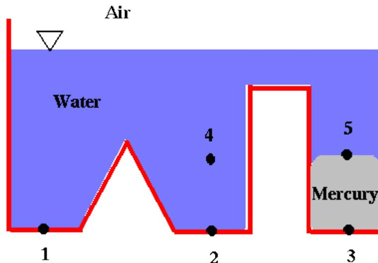
By this rule,  $p_1 = p_2$  and  $p_4 = p_5$  since these points are at the same elevation in the same fluid. However,  $p_2$  does not equal  $p_3$  even though they are at the same elevation, because one cannot draw a line connecting these points through the *same* fluid. In fact,  $p_2$  is *less than*  $p_3$  since mercury is denser than water.
