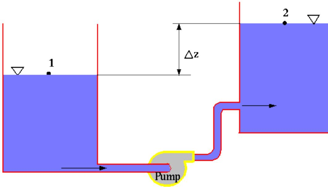
Again, the little upside-down triangle indicates a free surface, and means that the pressure there is atmospheric pressure,  $p_a$ . In other words, in this example,  $p_1 = p_a$  and  $p_2 = p_a$ . But since point 2 is higher in elevation than point 1, the local atmospheric pressure at 2 is a little lower than that at point 1. To be precise, our hydrostatics equation must be used to account for the difference in elevation between points 1 and 2:
