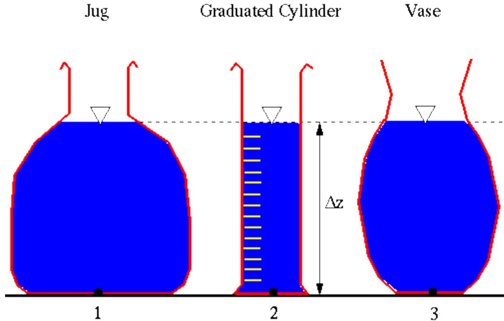
At first glance, it may seem that the pressure at point 3 would be greater than that at point 1 or 2, since the weight of the water is more "concentrated" on the small area at the bottom, but in reality, all three pressures are identical. Use of our hydrostatics equation confirms this conclusion, i.e.
