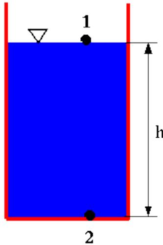
The little upside-down triangle indicates a free surface, and means that the pressure there is atmospheric pressure,  $p_a$ . In other words, in this example,  $p_1 = p_a$ . To find the pressure at point 2, our hydrostatics equation is used:
