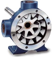
Internal gear pumps are exceptionally versatile. While they are often used on thin liquids such as solvents and fuel oil, they excel at efficiently pumping thick liquids such as asphalt, chocolate, and adhesives. The useful viscosity range of an internal gear pump is from 1cPs to over 1,000,000cP.
