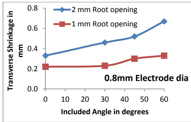
Figure 3: Variation of transverse shrinkage with included angle for 0.8 mm electrode diameter in double V groove butt welded joints.
