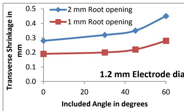
Figure 2: Variation of transverse shrinkage with included angle for 1.2 mm electrode diameter in V groove butt welded joints.
