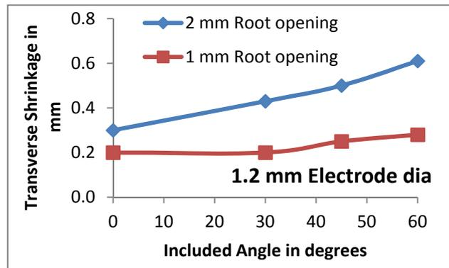
Figure 4: Variation of transverse shrinkage with included angle for 1.2 mm electrode diameter in double V groove butt welded joints.
