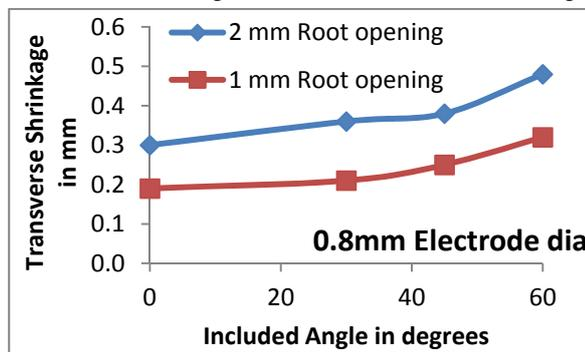
Figure 1: Variation of transverse shrinkage with included angle for 0.8 mm electrode diameter in V groove butt welded joints.
