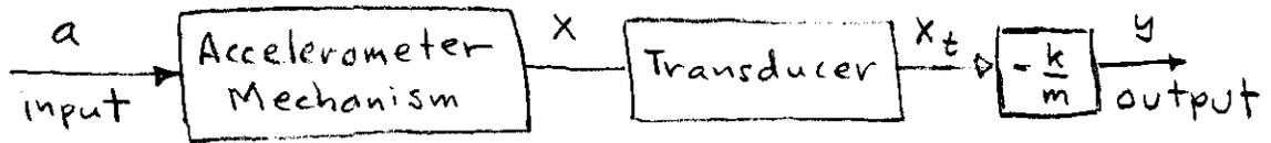
Note in particular that if the vehicle acceleration is constant then the steady state output is constant, thus producing an indication of that acceleration.
