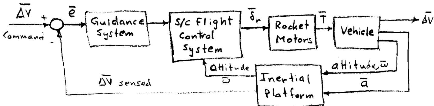
Note the inner loop that controls vehicle attitude and the outer loop that controls the velocity change imparted by the rocket motors. The inner loop utilizes both attitude and angular velocity measurements, from the inertial platform gyros, to stabilize and guide the vehicle. The outer loop utilizes integrated accelerometer outputs to achieve the desired velocity change.
