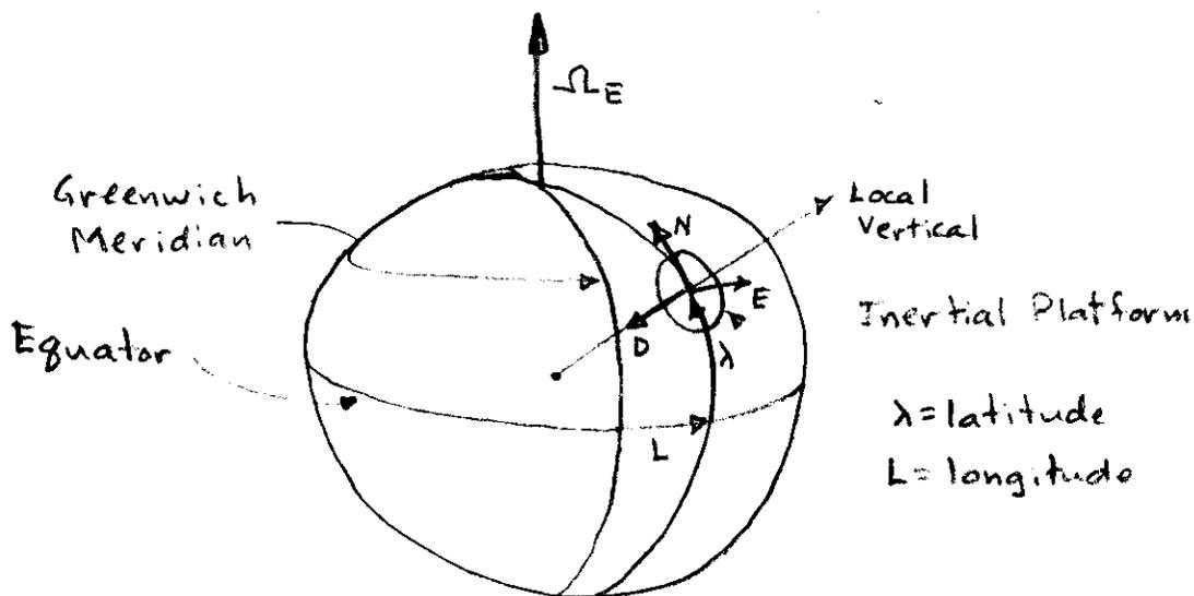
In effect the inertial platform provides a replica of the local horizon within the aircraft and serves as the reference for the horizontal situation indicator on the aircraft instrument panel. The inertial platform gimbals allow the inertial platform to remain stable, with respect to the local vertical, even as the vehicle may perform violent angular maneuvers about the stable inertial platform.
