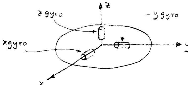
Applying torque to the gyro causes its spin vector (i.e., angular momentum vector) to move with respect to inertial space. Thus the inertially stabilized platform can be reoriented with respect to inertial space.
