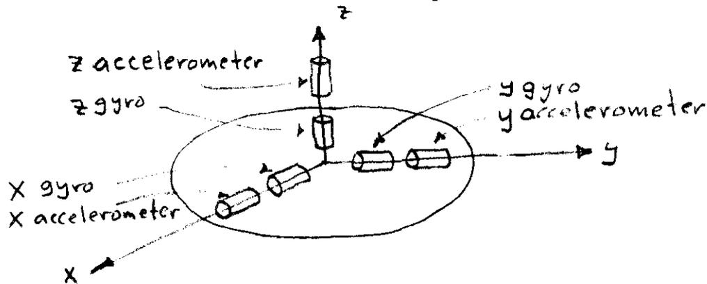
The three gyros stabilize the platform orientation so that it is stationary with respect to inertial space. Each gyro is responsible for stabilization about one axis. The stable platform holds the accelerometers fixed in space so that they can sense acceleration. The three components of acceleration are then integrated to estimate the change in vehicle velocity vector.
