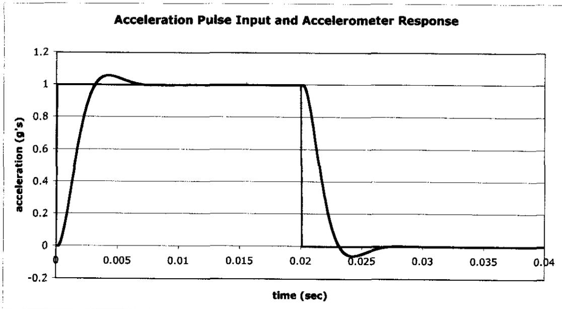
Commonly vehicle velocity is desired so the accelerometer output is integrated over time
