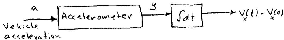
The following figure illustrates the vehicle velocity produced by the acceleration pulse shown above, compared with the time integral of the accelerometer output.
