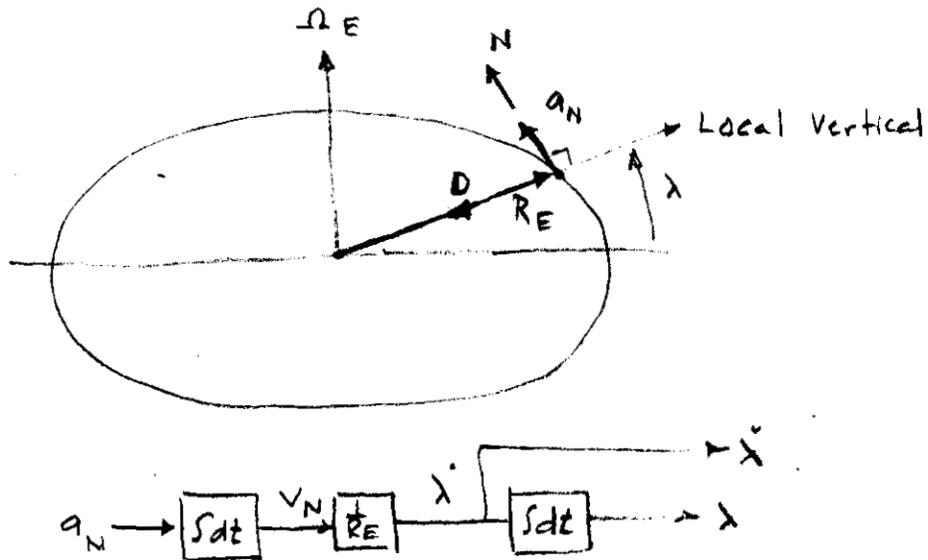
In addition, the attitude rate indication is used to torque the north and down gyros as indicated above. A similar function is performed on the east accelerometer outputs so as to maintain longitude.
