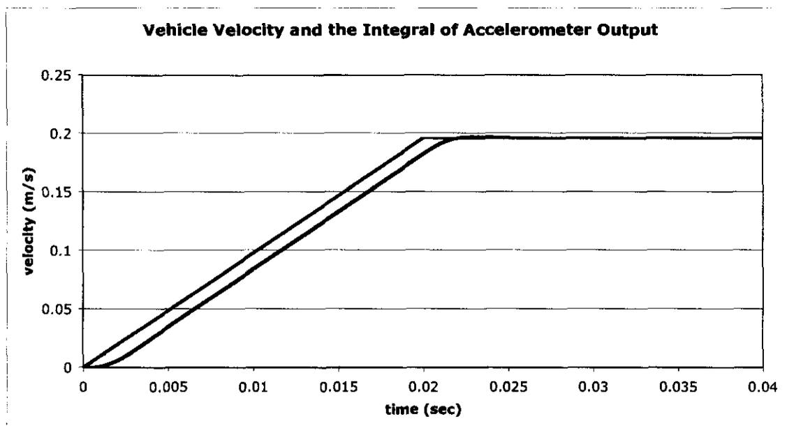
Note that, except for a small delay, the integral of the accelerometer output is a very good representation of vehicle velocity.
