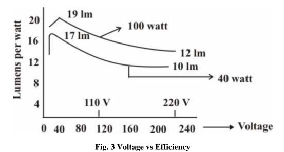
Fig. 3 shows variations of voltage with luminous efficiency for 40 W and 100W lamps. As may be observed for both the lamps variation in luminous efficacy between 200 - 240V is very little. It implies that small variations in voltage do not effect the light efficiency. Where as in the 110V region variation is significant though one gets higher efficacy compared to 220V region.
