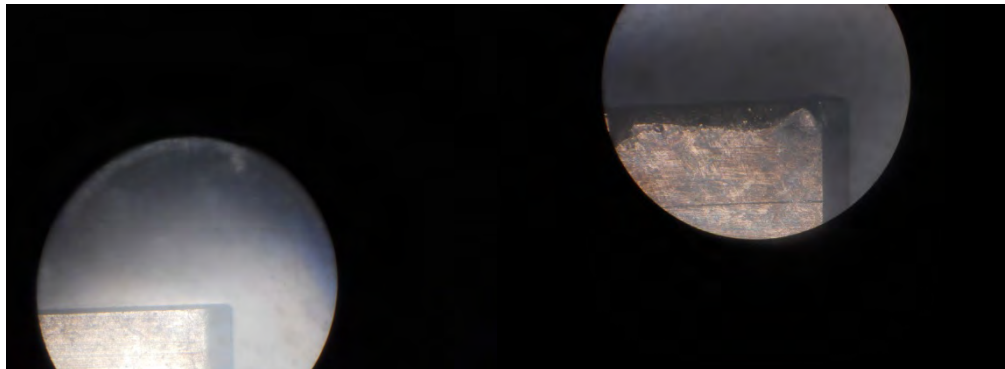
Fig. 16. Initial and final condition of tool wear
