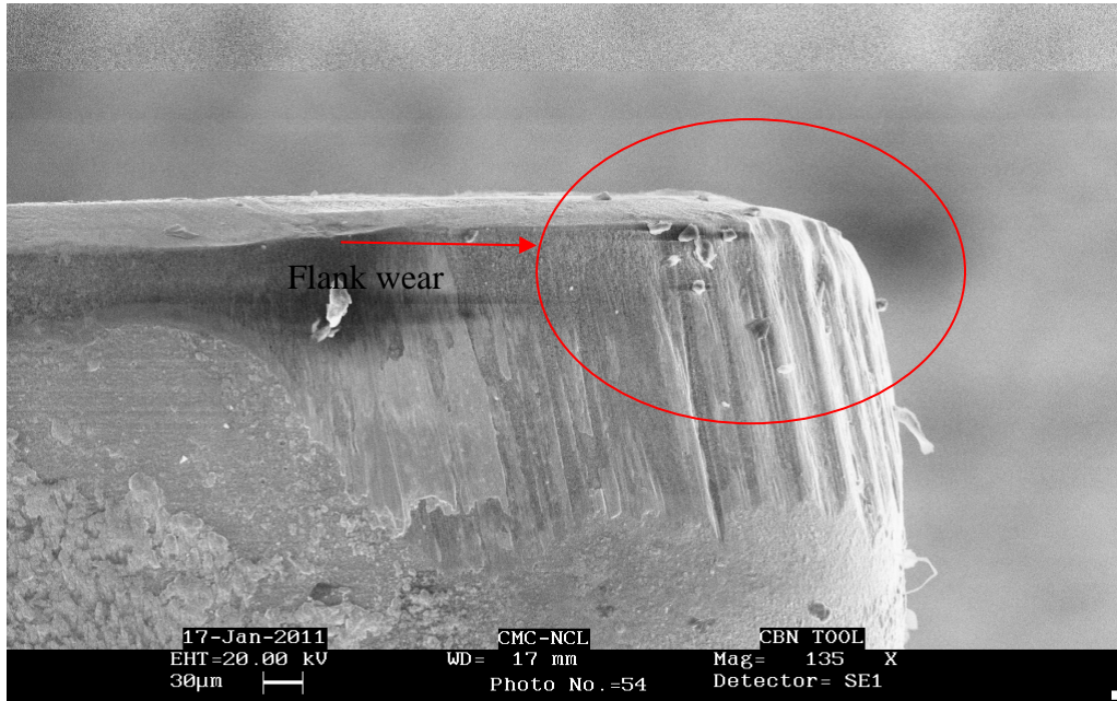
Fig. 17. SEM view of worn out insert (flank surface) after machining
