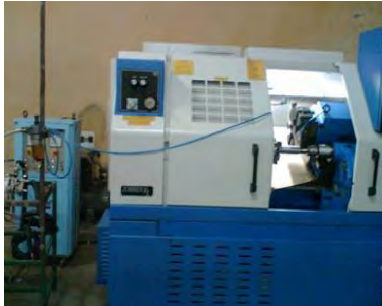
Fig.1. Experimental set up showing minimal cutting fluid delivery unit
