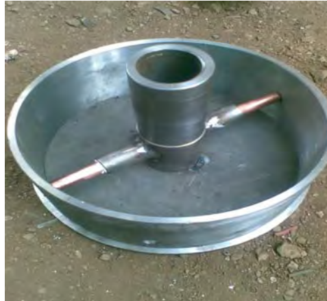
Fig 3.2: Heat pipe in horizontal orientation
