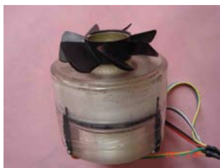
Fig.3: Passive maglev turbine model and its rotor position detection. The model has the same levitation structure as passive maglev pump, but 4- time larger dimension than the pump. 4 Hall sensors detect the position of the rotor. As the propeller is driven by a compressor to rotate, then the rotating speed will gradually decrease. It demonstrates the maximal ED is smaller than gap (0,15mm) when rpm is larger than 1800; and max. ED will reach
