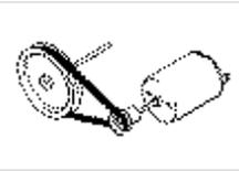
This arrangement can be used to either increase power, increase speed and to change direction of motion.
