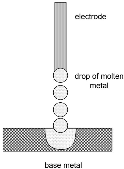
Fig. 8.3 (c) Schematic of spray metal transfer
