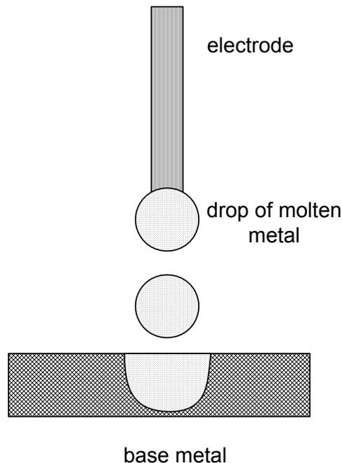
Fig. 8.3 (b) Schematic of globular metal transfer
