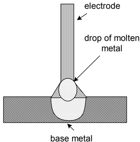
Fig. 8.3 (a) Schematic of short circuiting metal transfer
