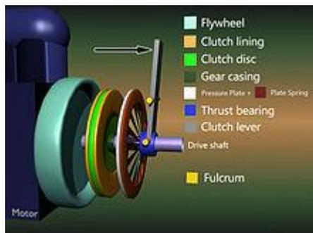
**Clutch** for a drive shaft: The clutch **disc** (center) spins with the flywheel (left). To disengage, the lever is pulled (black arrow), causing a white pressure plate (right) to disengage the green clutch disc from turning the drive shaft, which turns within the thrust-bearing ring of the lever. Never will all 3 rings connect, with no gaps.
