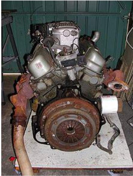
Rear side of a Ford V6 engine, looking at the clutch housing on the flywheel
