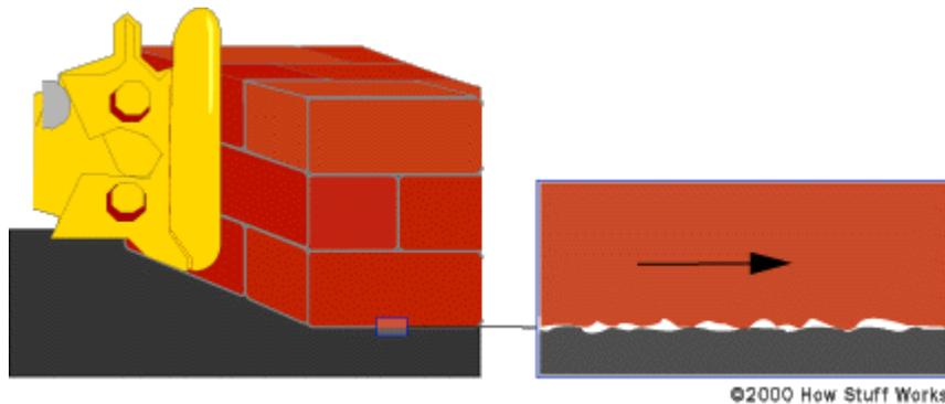
**Because friction exists at the microscopic level, the amount of force it takes to move a given block is proportional to that block's weight.**
