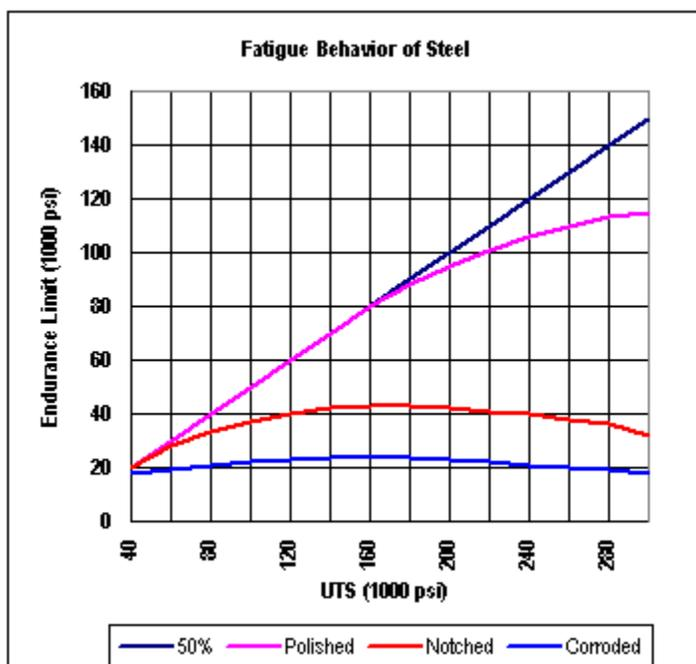
This plot illustrates the dramatic effect that fretting has on the fatigue life of steels. The line titled "Corroded" mirrors the shape of the "notched" curve, but is much lower. The corroded curve shows that, for a badly corroded surface (fretting, oxidation, galvanic, etc.) the endurance limit of the material starts at around 20 ksi for materials of 40 ksi **UTS** (50%), increases to about 25 ksi for
