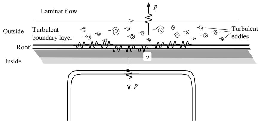
Figure 4.7 The pressure fluctuations generated by the turbulent vortices are responsible for noise both inside and outside of the vehicle. [1]
