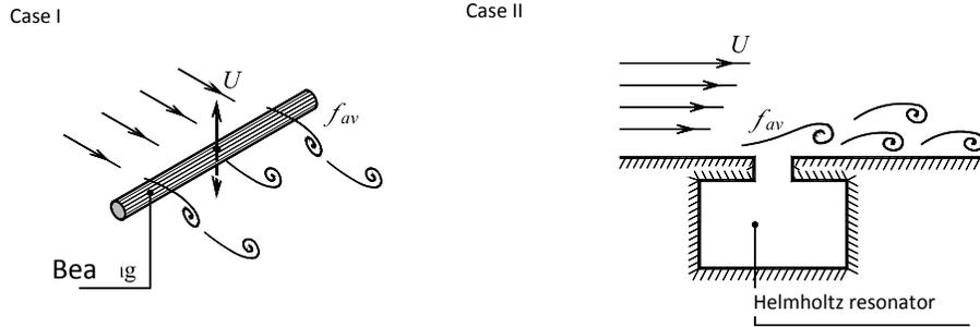
Figure 4.11 Two examples of how whistle tones can be generated in a flow field.
