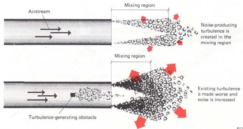
Figure 4.10 By reducing the velocity difference (gradient) in the mixing zone, the sound and vibration radiation of the jet can be reduced. (Picture: Asf, Bullerbekämpfung, 1977, Illustrator: Claes Folkesson) [1]
