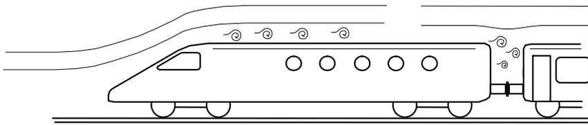
Figure 4.6 When vehicles move at high speeds, pressure fluctuations are generated, i.e., sound and vibration arises, due to the turbulent boundary layer of the flow field. [1]
