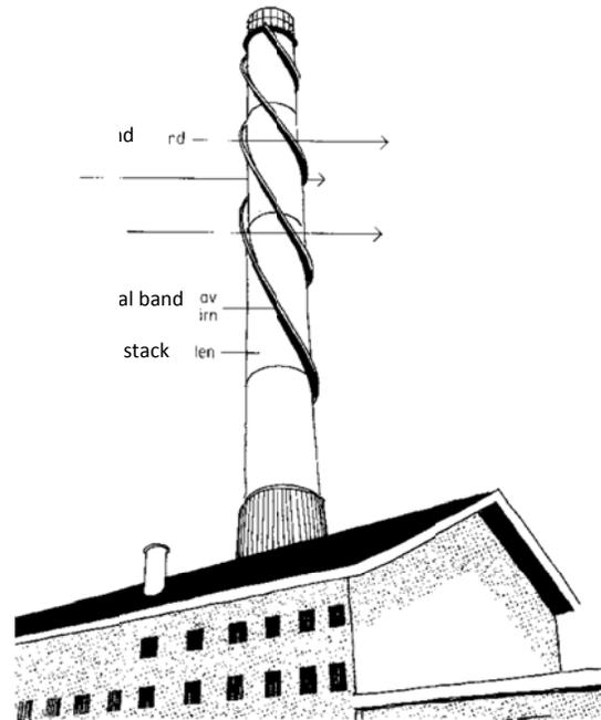
Figure 4.12 The whistling sound and vibration generated by a periodic vortex shedding from a smoke stack can be eliminated by wrapping the stack with a spiral band. That effectively disturbs the vortex generation. (Picture: Asf, Bullerbekämpning, 1977, Ill: Claes Folkesson) [1]
