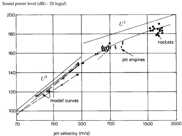
Figure 4.9 Velocity dependence of the sound and vibration generation from jet and rocket engines, from Chobotov & Powell, 1957. Note that the sound and vibration power is corrected for the size  $d$  of the sources by the scaling law given by equation (4.8).
