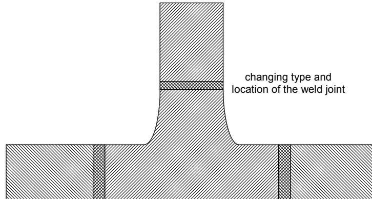
Fig. 30.2 Schematic diagram showing change on joint configuration from fillet to butt joints
