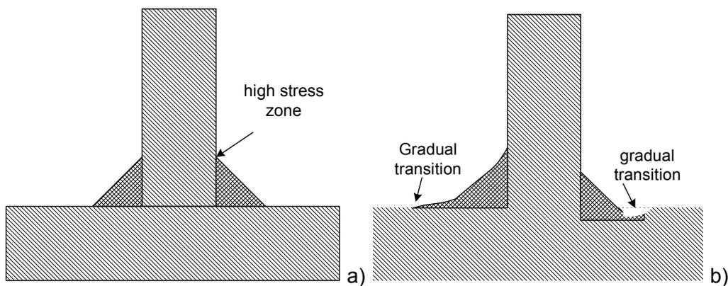
Fig. 30.1 Reducing stress concentration at toe of the weld a) toe with sudden change in cross section causing high stress concentration and b) providing some fillet at the toe of the weld by grinding
