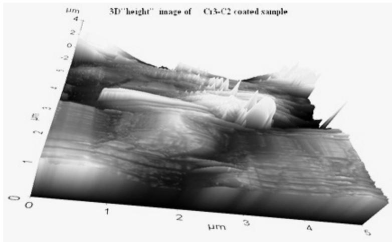
Figure -5 AFM 3-D “Height” Image of Cr<sub>3</sub>-C<sub>2</sub> coated sample
