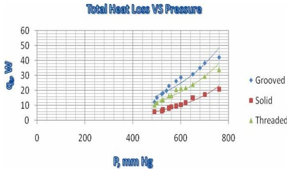
Fig. 15: Comparison of total heat loss by solid, grooved and threaded cylindrical fin at different pressure
