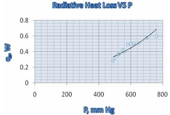
Fig. 13: Effect of pressure reduction on radiation from a threaded cylindrical fin
