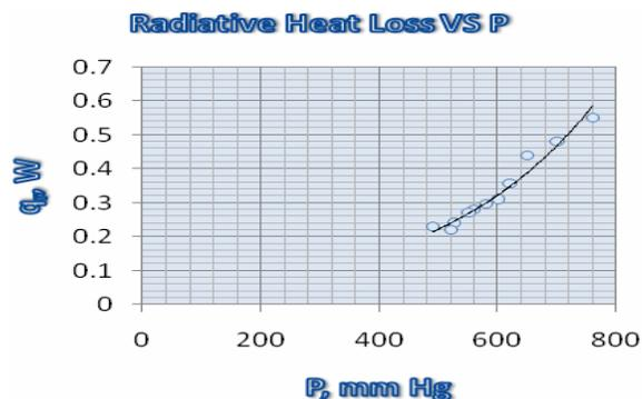
Fig. 5: Effect of pressure reduction on radiation from a solid cylindrical fin
