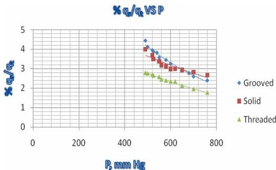
Fig. 16: Comparison of participation of radiation on total heat loss for solid, grooved and threaded Cylindrical fin with varying pressure.
