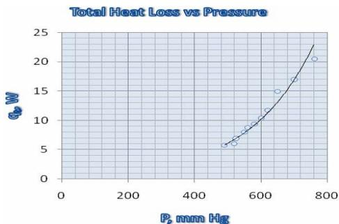
Fig. 3: Effect of pressure reduction on heat transfer from solid cylindrical fin
