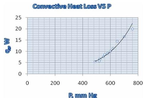
Fig. 4: Effect of reduction of pressure on convective heat loss by a solid cylindrical fin
