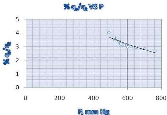
Fig. 6: Effect of pressure reduction on the percentage of radiation heat loss to total heat loss for solid cylindrical fin
