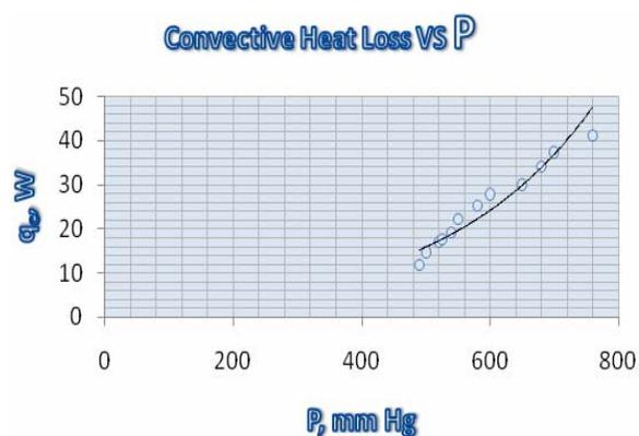
Fig. 8: Effect of reduction of pressure on convective heat loss by a grooved cylindrical fin
