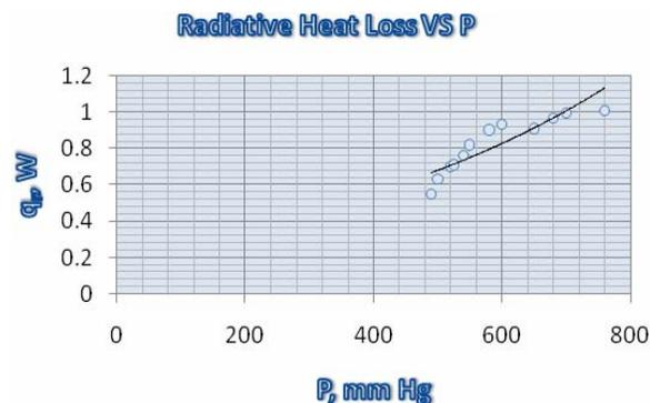
Fig. 9: Effect of pressure reduction on radiation from a grooved cylindrical fin
