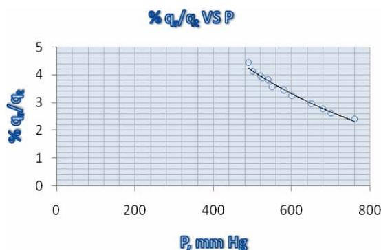
Fig. 10: Effect of pressure reduction on the percentage of radiation heat loss to total heat loss for grooved cylindrical fin
