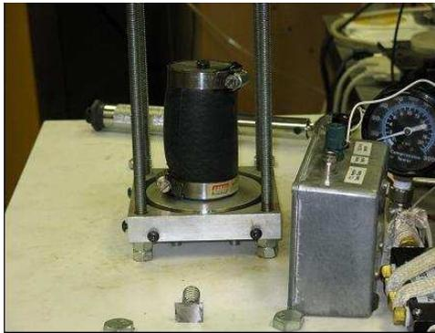
Fig. 4 Rubber bladder used to contain the propellant
