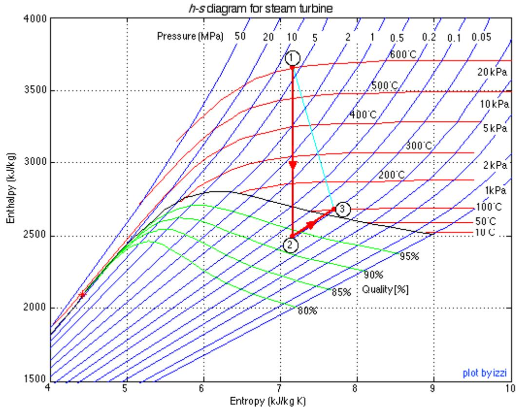
Notice from the h-s diagram that the heat exchanger temperature varies from the saturation temperature at 50 kPa (81°C) to 100°C at state (3). In order to accommodate that change we develop the differential form of the heat pump as follows:
