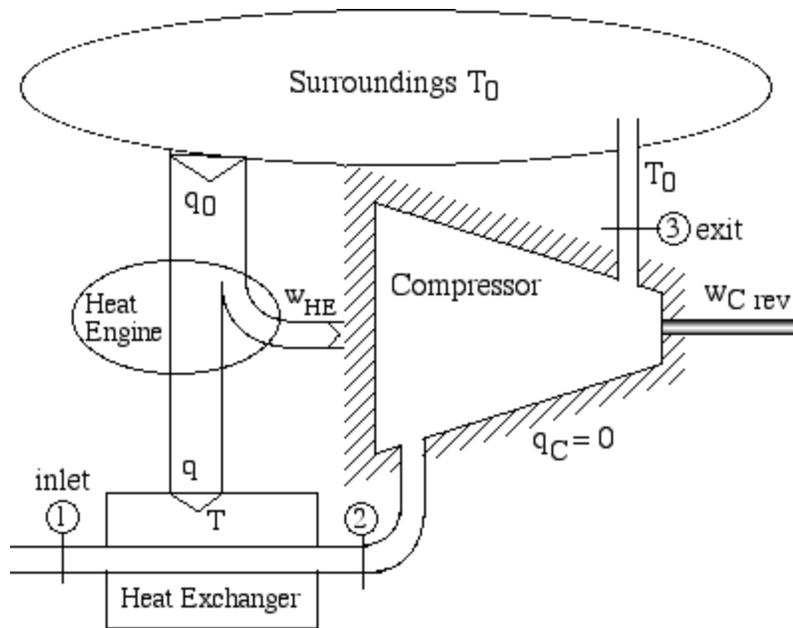
A typical  $h-s$  diagram for this system is shown below, in which we have used typical inlet conditions of 140kPa,  $-10^\circ\text{C}$  and exit conditions of 700kPa,  $60^\circ\text{C}$ . The reversible heat engine will provide extra work to drive the compressor, absorbing its heat from the environment temperature  $T_0$  while rejecting heat to the heat exchanger. The exit state (2) from the heat exchanger has been chosen such that the compression process (2) - (3) will be isentropic.
