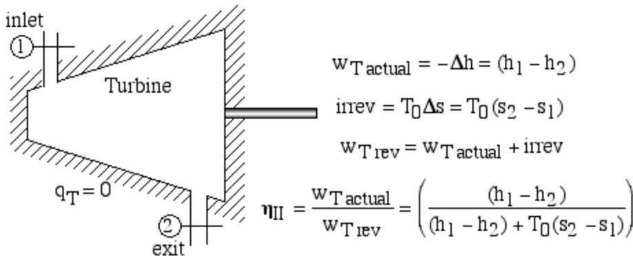
Once again, in an attempt to find some intuitive meaning to these equations we consider a reversible system having the same inlet and exit states as the actual turbine, comprising an isentropic turbine, a heat pump pumping heat from the surroundings to the heat exchanger in the exit stream. Note that as far as the adiabatic turbine is concerned we will assume that the surroundings temperature  $T_0$  is equal to the exit temperature.
