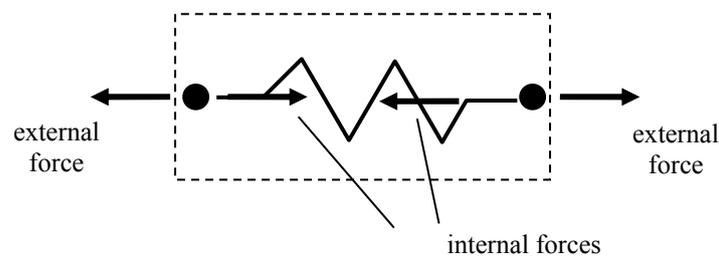
**Figure 8.1.6: external force pulling two molecules/particles apart**
