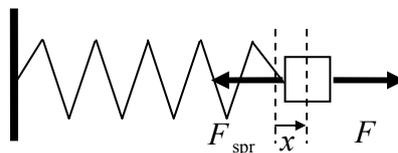
**Figure 8.1.2: a force extending an elastic spring**
