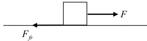
**Figure 8.1.4: Dragging a block over a frictional surface**
