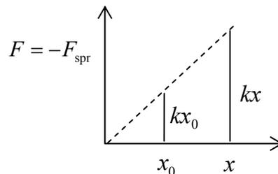
**Figure 8.1.3: force-extension curve for a spring** ■
