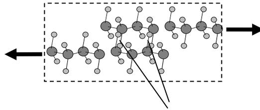
**Figure 8.1.7: external force pulling two molecules/particles apart**
