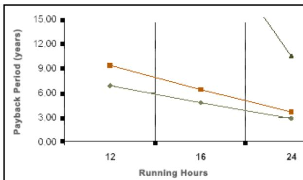
Fig. 6: Dual Fuel Operation Pay Back Period vs Running Hours
