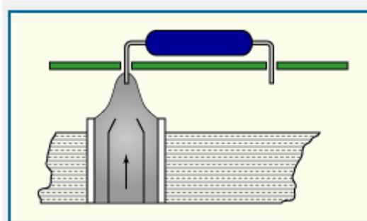
Figure 3: Mini-wave method for selective soldering
