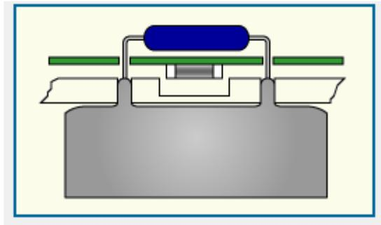
Figure 4: Stencil dip method for selective soldering
