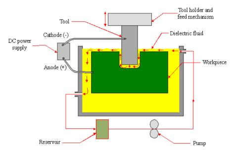
Figure 2: Schematic of EDM process
