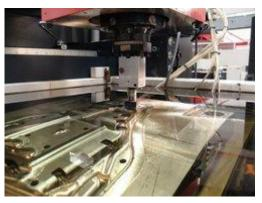
Figure 1: Electrical discharge machine
