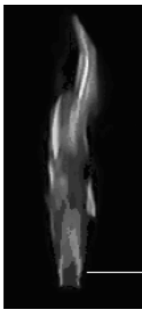
Fig.10. Tearing of flame base at higher air jet velocity close to the burner rim
