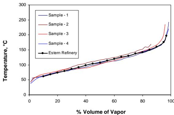
Figure 8(b). Distillation curve of Octane samples.
