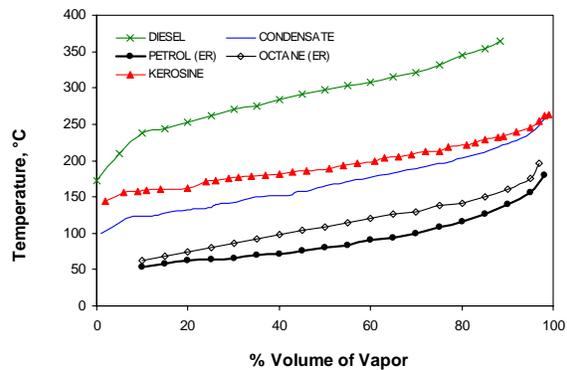
Figure 9(a). Distillation curve of different fuels samples.
