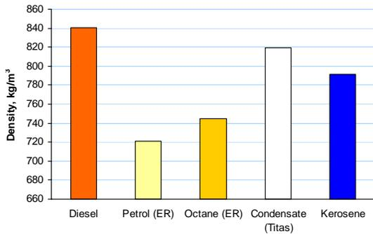
Figure 5. Comparison of densities measured of different types of colour coded fuels.
