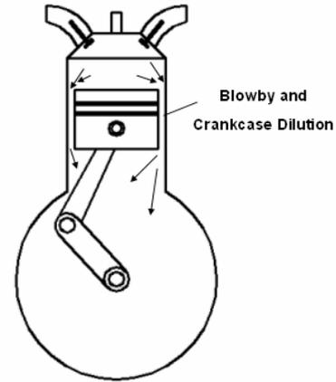
Figure 1. Crankcase dilution inside the engine
