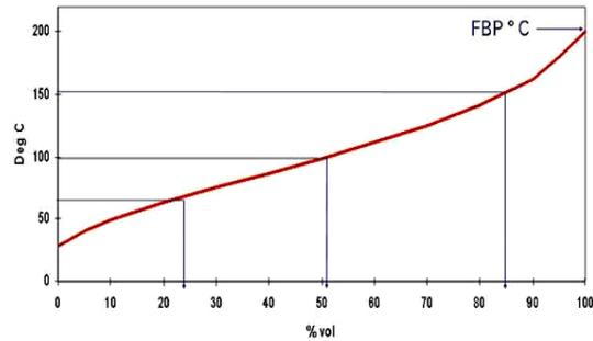
Figure 6. Typical distillation curve for gasoline.
