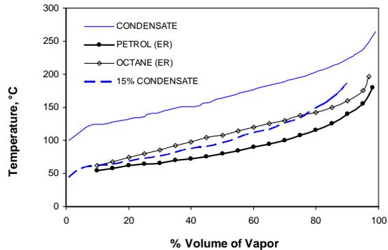
Figure 9(b). Distillation curve of 15% Condensate by volume with Petrol.
