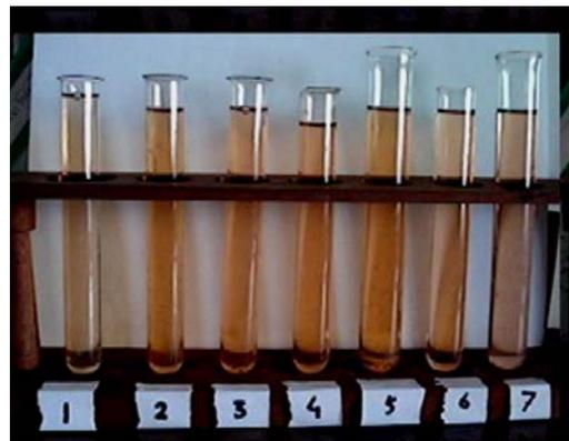
Figure 3(b). Colour comparison of octane samples, arrow sizes indicate colour darkness.
