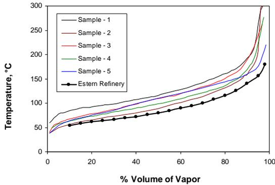
Figure 8(a). Distillation curve of Petrol samples.
