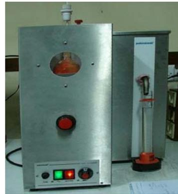
Figure 7. Distillation-Unit used, DU-4 Professional
