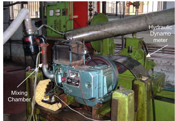
Fig. 2. The test engine coupled with a Dynamometer.
