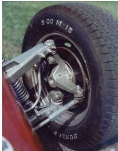
Suspension. On automobiles, disc brakes are often located within the wheel
