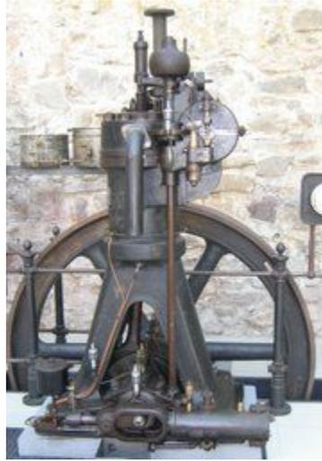
The diesel engine is one type of internal combustion engine; more specifically, it is a compression ignition engine, in which the fuel is ignited by being suddenly exposed to the high temperature and pressure of a compressed gas, rather than by a separate source of ignition, such as a spark plug, as is the case in of the gasoline engine.
