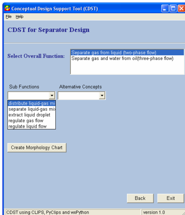
Fig. 6. Subfunctions for two phase separator
