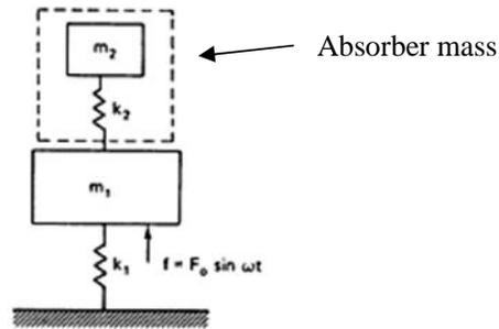
Fig. 7.9 Vibration absorber
