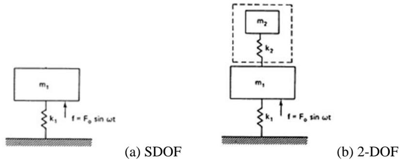
Fig. 7.10 Mass addition as vibration absorber
