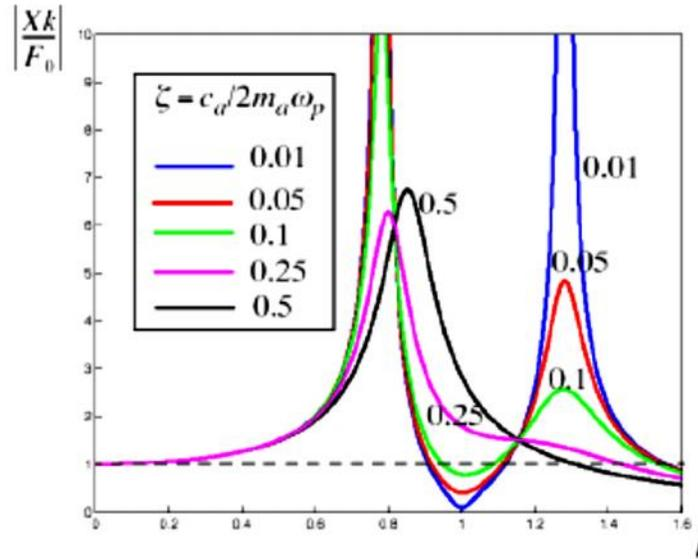
Fig. 7.12 Variation of amplitude with damping ratio
