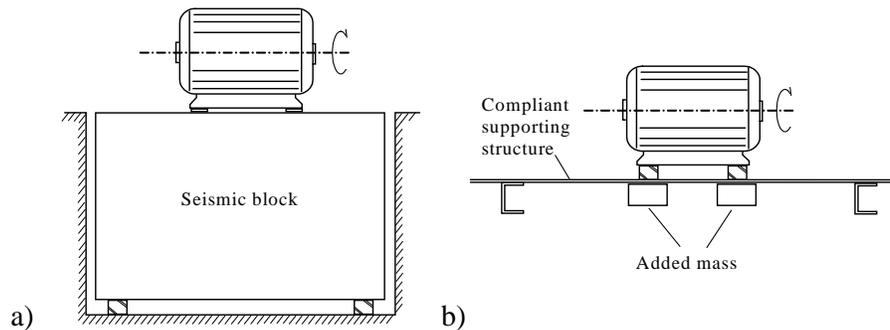
**Figure 7.13** Blocking masses, preferably in combination with elastic elements, give very good vibration isolation and are frequently used in practice. a) Seismic block. b) Added mass at a compliant point. [1]
