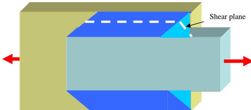
**Figure 3: Design of a parallel fillet joint**
