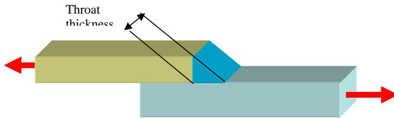
Figure 10.4.2: Design of a single transverse fillet
