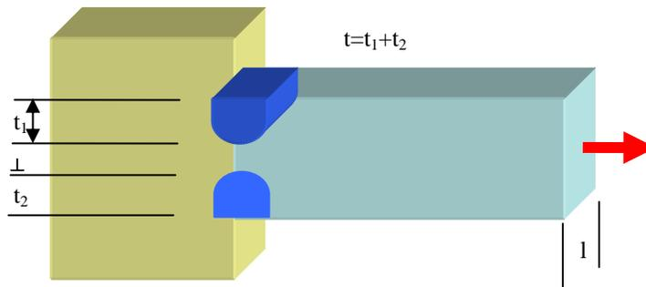
Figure 10.4.1: Design of a butt joint
