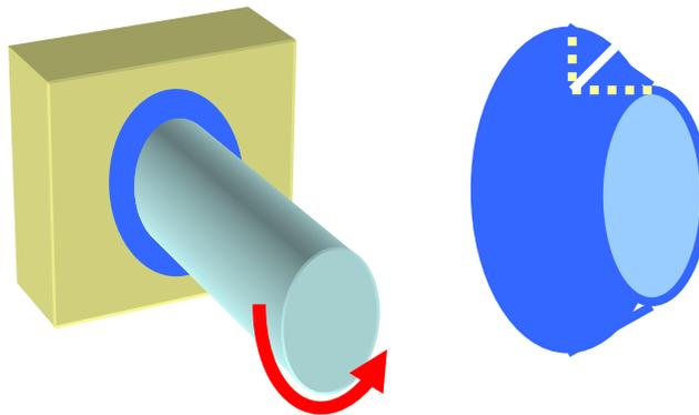
**Figure 10.4.5: Design of a fillet weld for torsion**
