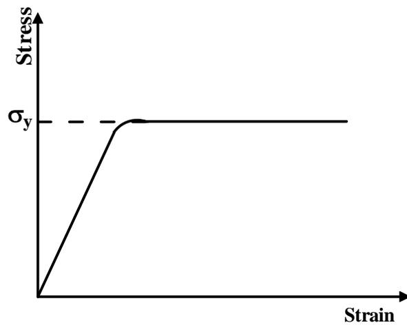
3.1.3.1F- (d) Stress-strain diagram for an elastic – perfectly plastic material.
