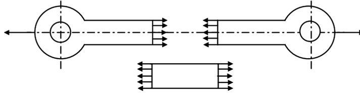
**3.1.1.1A- Stresses developed in a link subjected to uniaxial loading**
