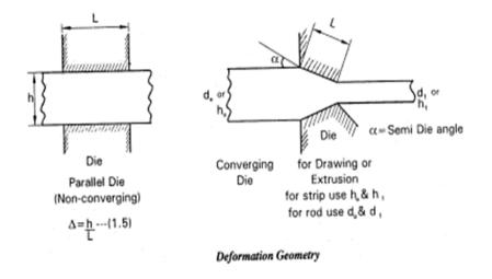
Most of the deformation processes require the material to flow through an opening or a converging channel called as die.
