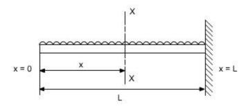
$$\begin{aligned} S.F|_{x=x} &= -w \\ B.M|_{x=x} &= -w.x. \frac{x}{2} = w \left(\frac{x^2}{2}\right) \\ \frac{M}{EI} &= \frac{d^2y}{dx^2} \\ \frac{d^2y}{dx^2} &= -\frac{wx^2}{2EI} \\ \int \frac{d^2y}{dx^2} &= \int -\frac{wx^2}{2EI} dx \\ \frac{dy}{dx} &= -\frac{wx^3}{6EI} + A \\ \int \frac{dy}{dx} &= \int -\frac{wx^3}{6EI} dx + \int A dx \\ y &= -\frac{wx^4}{24EI} + Ax + B \end{aligned}$$
