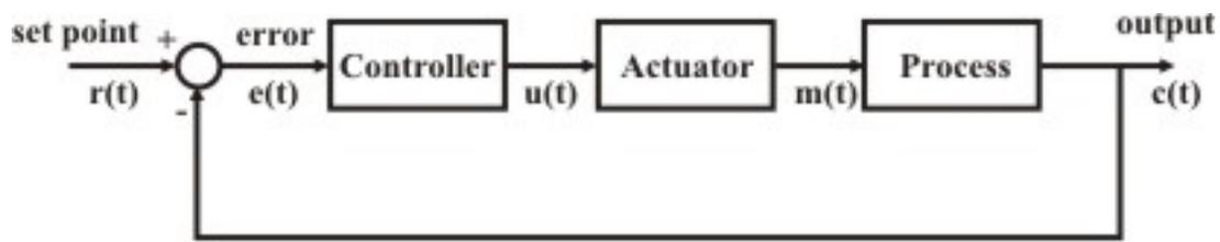
Fig. 1 Closed loop system.
