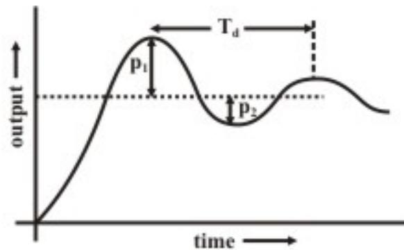
Fig. 5 Controller tuning using damped oscillation technique.
