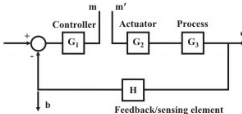
Fig. 2 Reaction curve technique for controller tuning.
