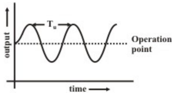
**Fig. 4 Controller tuning continuous oscillation mode.**
