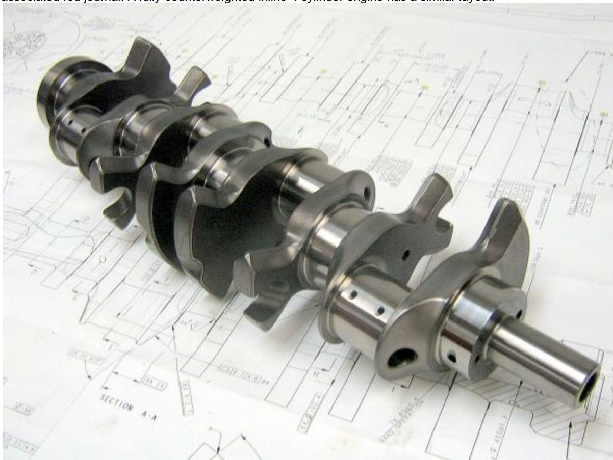
Figure 2 Single-Plane V8 Crankshaft (Courtesy of Bryant Racing)
