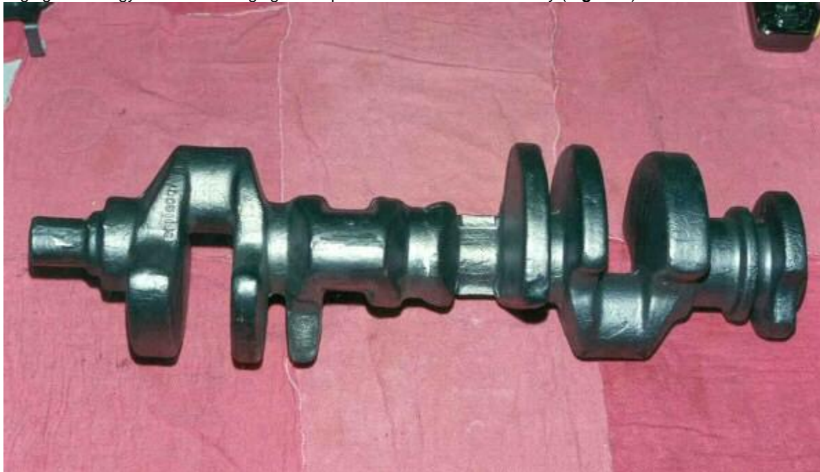
Figure 3 Two-Plane V8 Crankshaft Raw Forging
