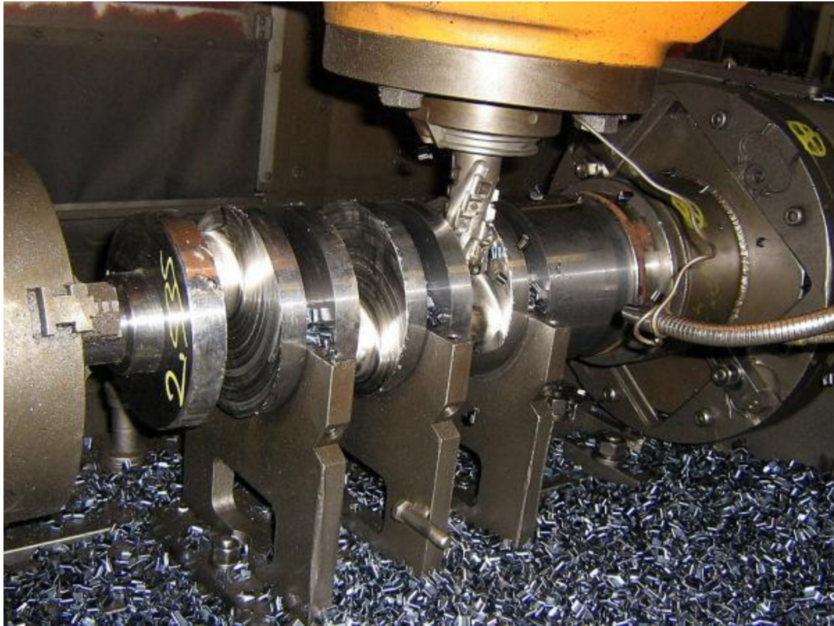
Figure 4 Billet Crankshaft Machining (Courtesy of Bryant Racing)
