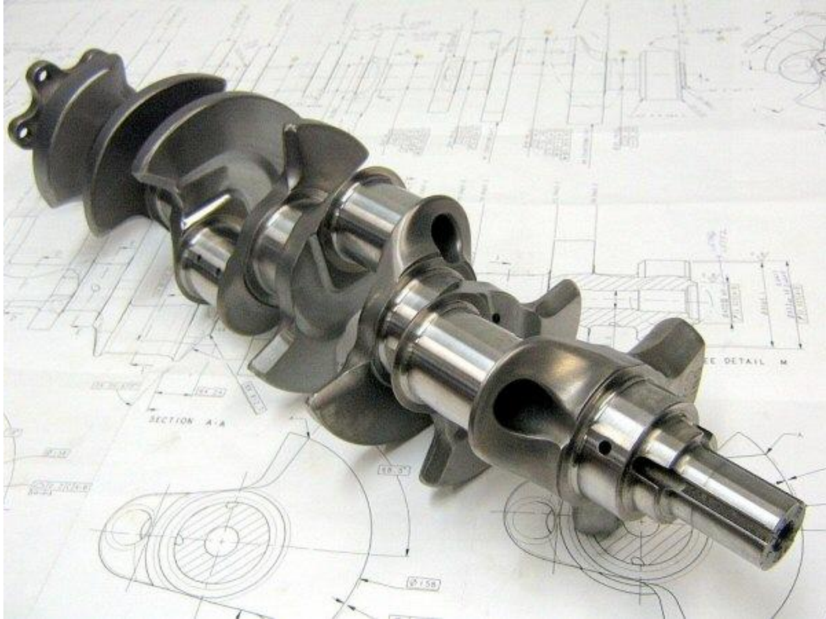
Figure 9 Fully-Counterweighted V8 Crank (Courtesy of Bryant Racing)
