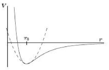
If the total energy is low enough so that the motion is restricted to the region where the curve is nearly parabolic, the system will behave like a harmonic oscillator. If V(r) is well behaved and has a minimum at
