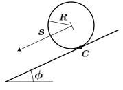
Conservation of energy implies that  $T+V = T_{initial} + V_{initial}$ . Initially, the kinetic energy is zero,  $T_{initial} = 0$ . Thus, for a later time, the kinetic energy is given by
