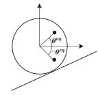
In order to study the stability of the equilibrium points, we need to determine whether the potential energy is a maximum or a minimum at these points. Since  $d^2V/d\theta^2 = -mgd\sin\theta$ , we have that when  $\theta^{eq.} < 0$ , then  $d^2V/d\theta^2 > 0$  and the potential energy is a minimum at that point. Consequently, for  $\theta^{eq.} < 0$ , the equilibrium is stable. On the other hand, for  $\theta^{eq.} > 0$ , the equilibrium point is unstable.
