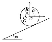
Since gravity is the only external force acting on the cylinder that is capable of doing any work, we can examine the equilibrium and stability of the system by considering the potential energy function. We have  $z_C = z_{C0} - R\theta \sin \phi$ , where  $z_{C0}$  is the value of  $z_C$  when  $\theta = 0$ . Thus, since d = |CG|, we have,
