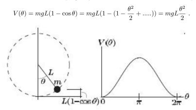
For small amplitude motions about  $\theta = 0$ , both the displacement  $\theta$  and the velocity are sinusoidal in time. As potential energy increases, kinetic energy decreases. Thus the minimum of V occurs at the maximum of T. The total energy is constant. The maximum value of kinetic energy is given by
