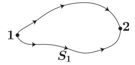
In one dimension any force which is only a function of position is conservative. That is, if we have a force, F(x), which is only a function of position, then F(x) dx is always a perfect differential. This means that we can define a potential function as
