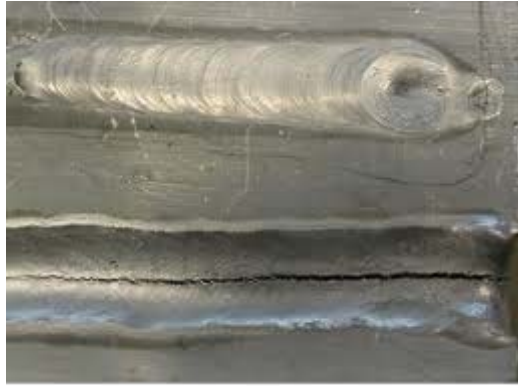
Fig. 38.3 Solidification cracking in aluminium weld
