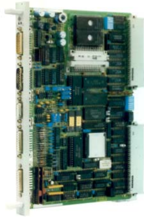
Fig. 24.10 A typical PLC Function module for Axis Control in a CNC
