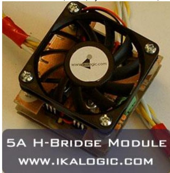
*In this article, I am going to show you how to build a relatively High power H-bridge motor controller (which is the most common way to control DC motors) **With cheap TIP transistors.***
