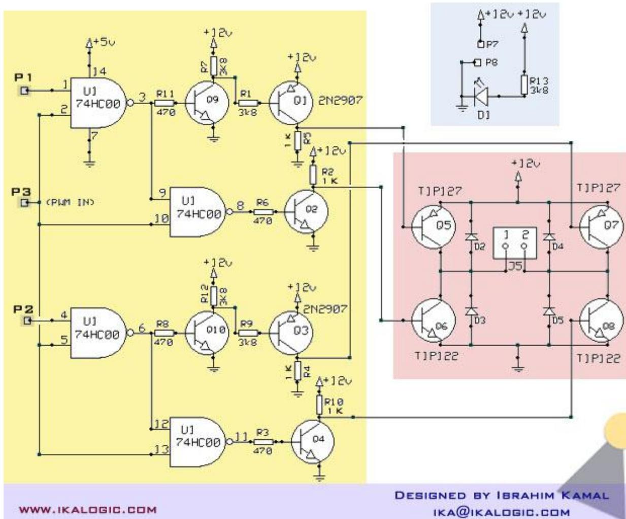
Note: Any transistor that is not labeled in the schematic, is a 2N2222 BJT
