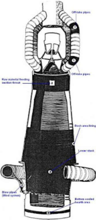
Fig: Typical areas of a Blast Furnace
