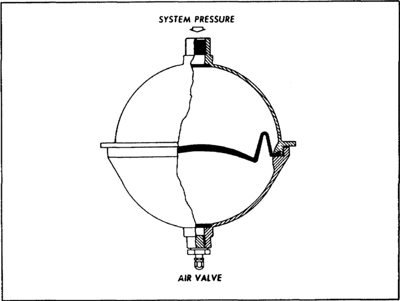
Figure 1-10. Diaphragm Accumulator.
