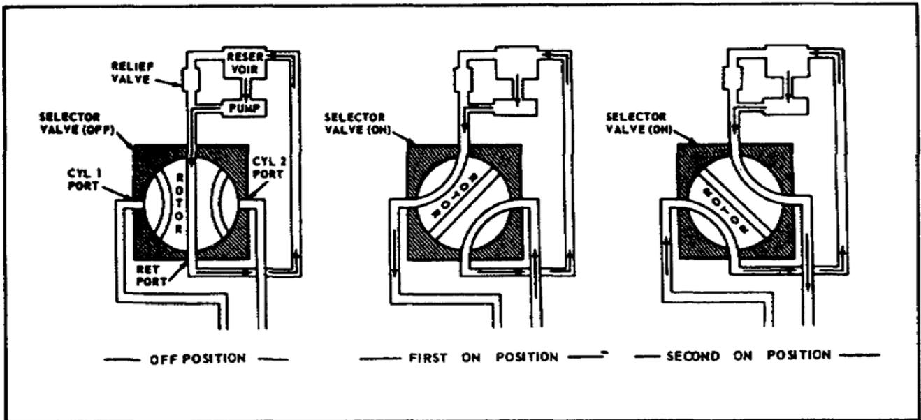
Figure 2-5. Typical Open-Center Rotor Selector Valve.
