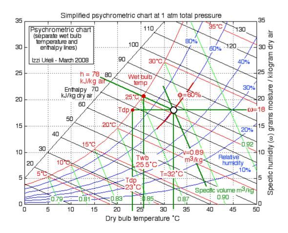
**Solved Problem 10.2:** Assume that the outside air temperature is 8°C. If the air in a room is at 25°C with a relative humidity  $\varphi = 40\%$ , use the psychrometric chart to determine if the windows of that room which are in contact with the outside will become foggy.
