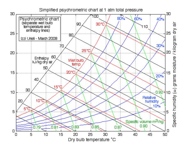
The four equations highlighted above were programmed in MATLAB and used to plot the simplified psychrometric charts shown above. Refer to the link: **MATLAB program for plotting a Simplified Psychrometric Chart**
