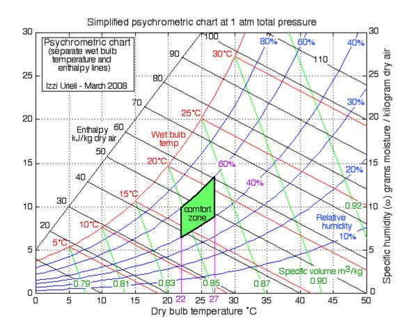
**Solved Problem 10.3:** Outside air at 35°C and 60% relative humidity is to be conditioned by cooling and heating so as to bring the air to within the "comfort zone". Using the Psychrometric Chart neatly plot the required air conditioning process and estimate (a) the amount of moisture removed [11.5g-H20/kg-dry-air], (b) the heat removed [(1)-(2),  $q_{cool} = 48$ kJ/kg-dry-air], and (c) the amount of heat added [(2)-(3),  $q_{heat} = 10$ kJ/kg-dry-air].
