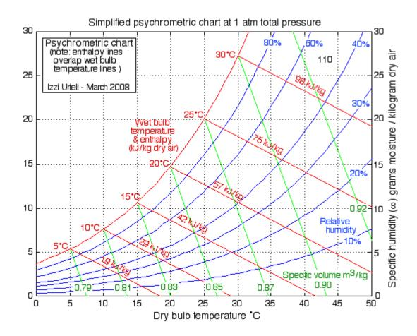
The basic information used to construct the chart is the water vapor saturation data (Tsat, Pg) which is obtained from steam tables over the range from Tsat =  $0.01^{\circ}$ C through 50°C. The specific humidity  $\omega$  is then evaluated using the relative humidity  $\phi$  as a parameter to produce the various relative humidity curves (blue lines) as follows:
