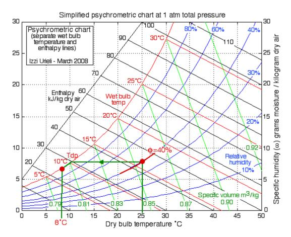
The air in contact with the windows will become colder until the dew point is reached. Notice that under the conditions of 25°C and 40% relative humidity the dew point temperature is slightly higher than 10°C, At that point the water vapor condenses as the temperature approaches 8°C along the saturation line, and the windows will become foggy.
