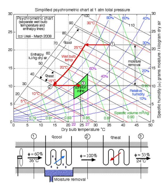
**Solved Problem 10.4:** Hot dry air at 40°C and 10% relative humidity passes through an evaporative cooler. Water is added as the air passes through a series of wicks and the mixture exits at 27°C. Using the psychrometric chart determine (a) the outlet relative humidity [45%], (b) the amount of water added [5.4g-H20/kg-dry-air], and (c) the lowest temperature that could be realized [18.5°C].
