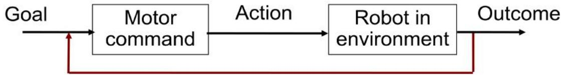
Fig. 3.1 (a) Scheme of feedback control
