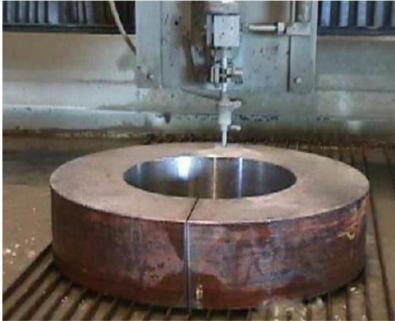
Figure 16: Abrasive water jet cutting
