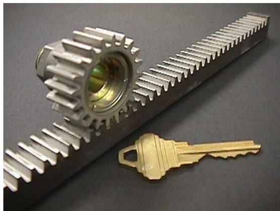
Figure 17: Steel gear and rack cut with an abrasive water jet
