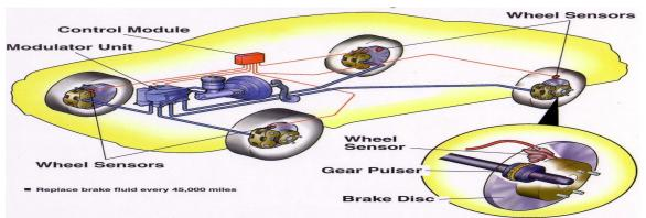
The EBCM then looks at the speed sensor signal from the affected wheel again. If that wheel is still decelerating, it opens the solenoid valve for that circuit. Once the affected wheel comes back up to speed, the EBCM returns the solenoid valves to their normal condition allowing fluid flow to the affected brake. Loss of hydraulic fluid in the brake master cylinder will disable the anti-lock system.
